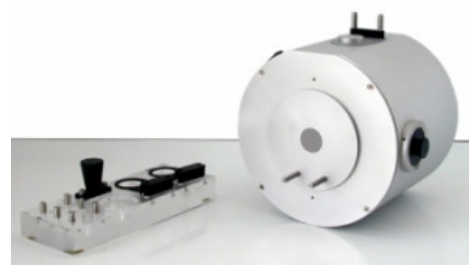
UPK-150 Integrating Sphere in Custom Design for Photoluminescence Measurements
