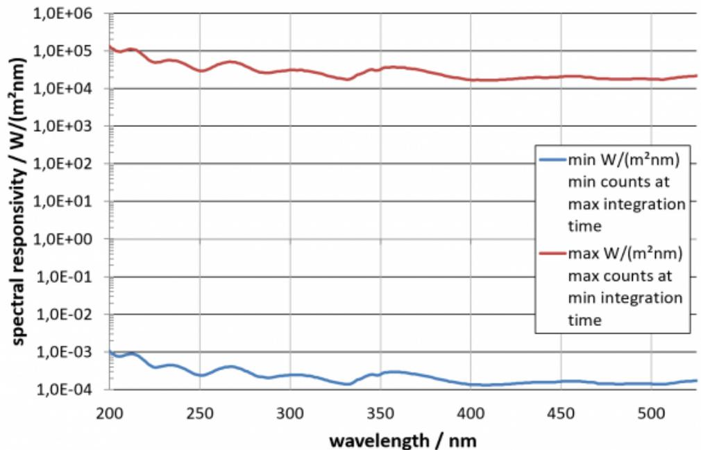
typical spectral responsivity BTS256-UV-4 (standard calibration 225 nm to 525 nm):
