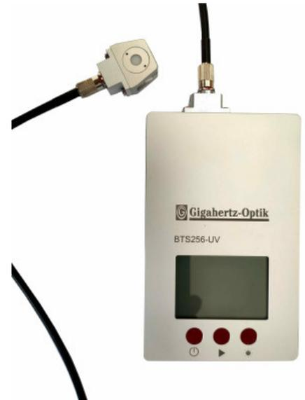
BTS256-UV-4 hand-held measuring device with flexible detector head.
