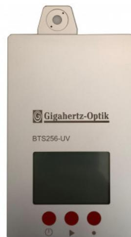
BTS256-UV-3 for measurement in direction of the upper side of device
