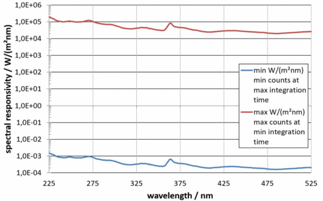
typical spectral responsivity BTS256-UV-2 and BTS256-UV-3 (standard calibration 200 nm to 525 nm):
