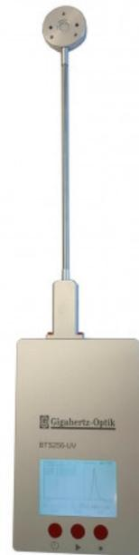
BTS256-UV-1 hand-held with safety distance to UV radiation
