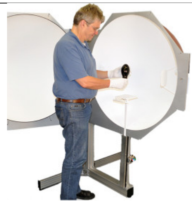
BTS256-LED Tester with 1m diameter integrating sphere
