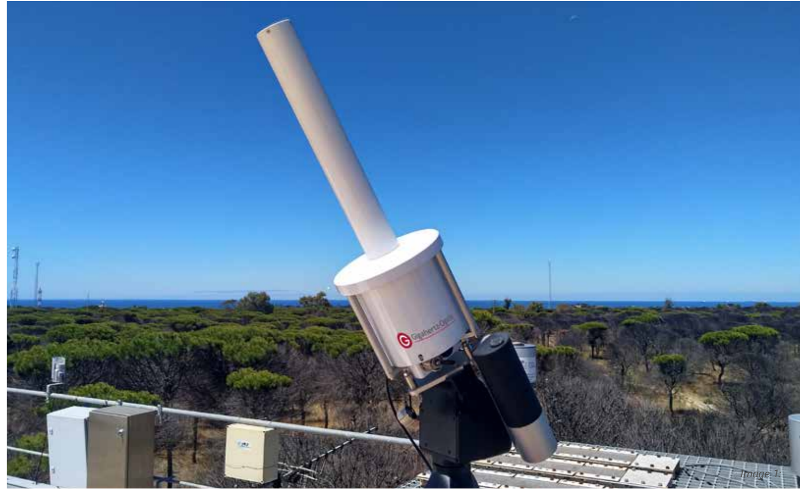
Image 1: CCD array spectroradiometer with sun tracker for recording the total ozone column (TOC) by direct measurements of solar radiation in the UV spectral range
