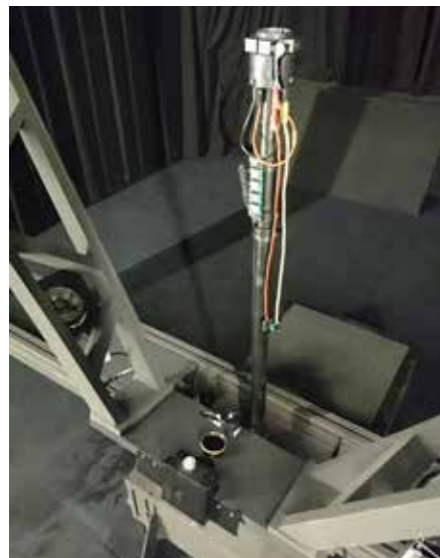
Image: BTS2048-VL-TEC retrofit into a goniometer system
