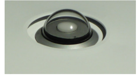
Entrance optic is blow-dried by warm air to prevent dirt, rain or snow
