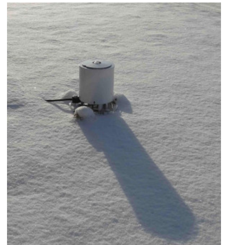
The BTS2048-IR-WP spectroradiometer with thermoelectrically cooled array detector
