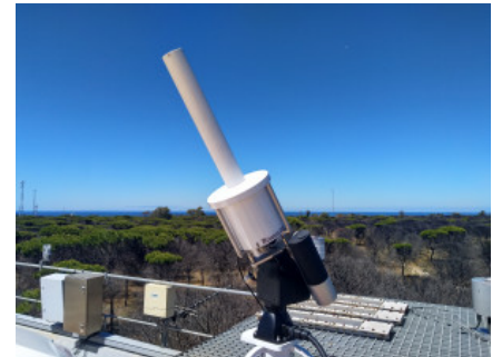
SUT-1711 equipped with BTS2048-UV-S-WP and tube for direct sun measurement
